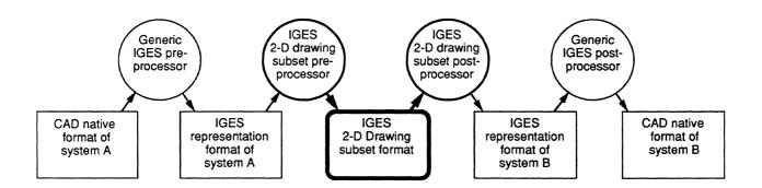
NOTE: The IGES application (the 2-D drawing subset) is an optional further step in the processing of the originating source file which, in addition to being converted from its native structure to a generic IGES structure, is also 'flavoured' to match the application subset.
